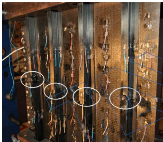
(a) 筋条断裂和脱黏
